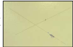
GALVANNEAL SHEET STEEL with our powder coat finish after a 336 hour salt spray test.
