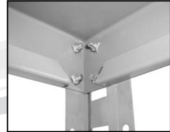
Top and bottom shelves are triple flanged at all four sides and bolted to angle posts at all four corners for maximum rigidity, durability and stability.
